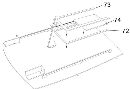
Glue the lower hatch frame 72 onto the roof with its rear edge flush with the rear edge of the roof.
