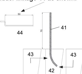
Bend a radius to the lower end of rudder shaft 41 to fit into rudder blade 42 and glue it in with Epoxy.
