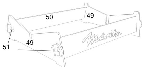
Stick together the boat stand with parts 49 to 51 as shown on the drawing.
