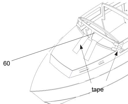
Place the front window 60 with tape centred on the cabin roof. Fix with some tape to the cabin sides and glue.
