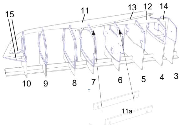
For keeping the distance correctly, stick distance pieces 11a onto bulkhead 6 and 7 near to the keel. **Do NOT glue them.**
