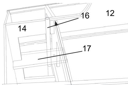
The ruder tube should protrude about 4 mm out of the keel.
