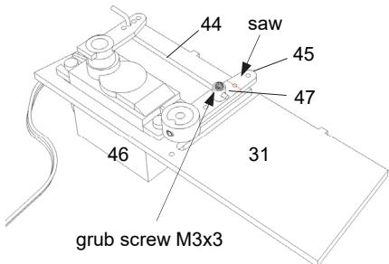
Drill open the next hole to 2 mm.
