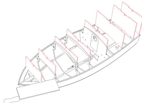
Turn the boat around to glue everything from inside. The hull sides should only be clamped to the stringers, not to the bulkheads, to avoid dents in the hull by shrinking of glue.
