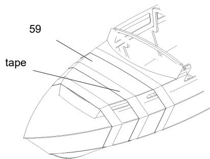
Turn the boat upside down to avoid that glue drops down into the hull.
