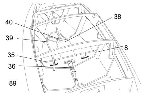
Glue motor mount with adapted motor and shaft as one unit onto the floor of the hull.
