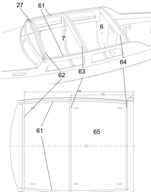
Place two strips 61 into the upper cut outs of bulkheads 6, 7 and 27.
