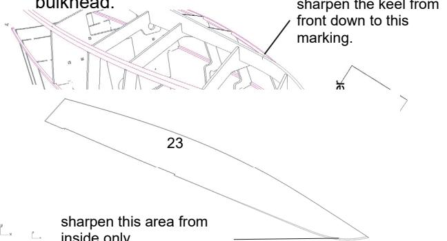
check clearly to sharpen from the inside, which also shows the markings for easy bending. Further to the rear you only need to sand the longitudinal side to fit next to the keel.
