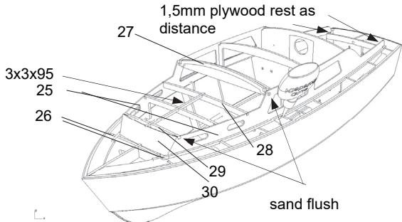
Place cabin front 30 down onto the centre hook and fix with tape to the cabin sides. Then glue.
