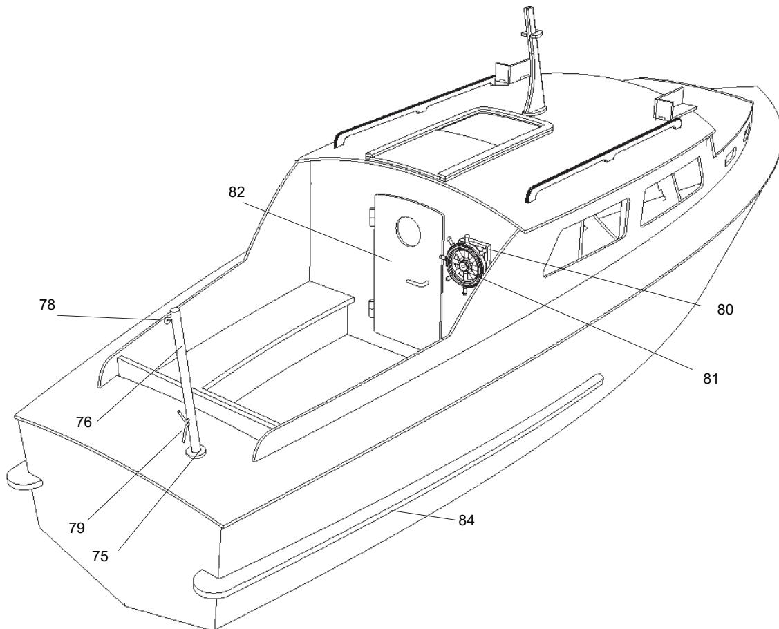
Glue two steering wheel box parts 80 together and onto the right rear wall of the cabin onto the hole.
