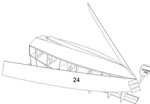
After the glue has set, give wood glue only to the stringers. Bend both sides equally over the frame and fix.
