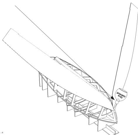
After the glue is fixed, bend both floor plates down to the bulkheads and stringers. Fix the plates with big clamps onto the bulkheads.
