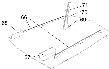
Glue the mast 70 into the mast base 69.
