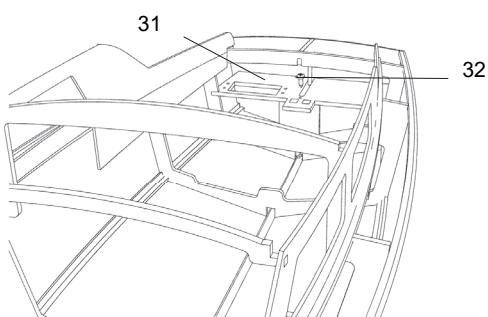
Place the servo tray 31 into the slots of bulkhead 3 and 4.
