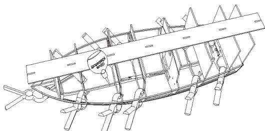
Tighten the gap between keel and floor from outside with tape. Now glue the plates from inside to the stringers and the keel. Glue to the frames later.
