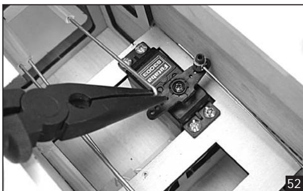
Cut and bend "L" the rudder pushrod.
