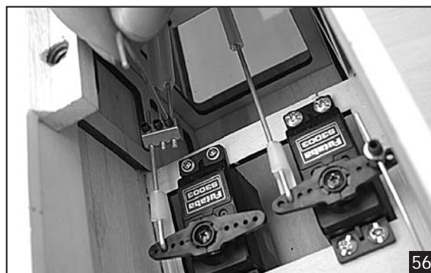
Install the elevator pushrod and secure it.
