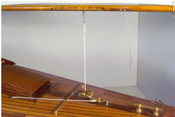
Installing the headsail winch
