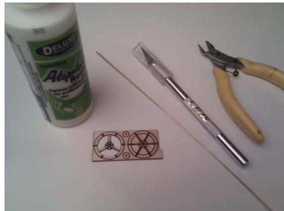
For this assembly fo the steering wheel you will need the small laser sheet, 12 cm of brass wire 1 mm, and white glue or Aliphatic glue, a mod-elling knife, a wire cutter and some sand pa-per.
