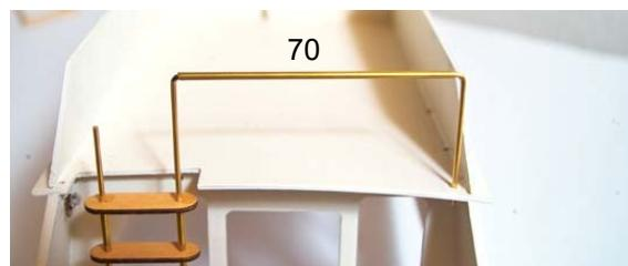
Make the lower rail from two split pins (71) and the tube (70).
