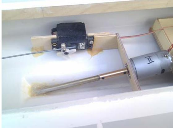
Now fix the tube and the motor mount with UHU Plus Acrylit inside the hull and fill the end of the hull around the shaft with glue that it is water tight.
