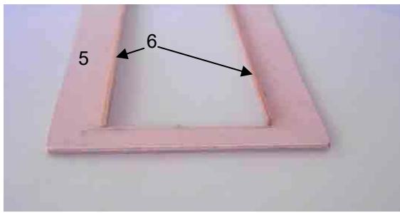
Now the coaming strips (10 to 13) have to be glued vertical onto the strips, that they are flush on the underside and protruding on the upper side. The superstruter will stand over this and so no water can come into the model hull.
