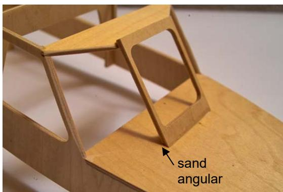
The front windows at the side have to be bevelled at the lower edge and at the edge to the centre window.
