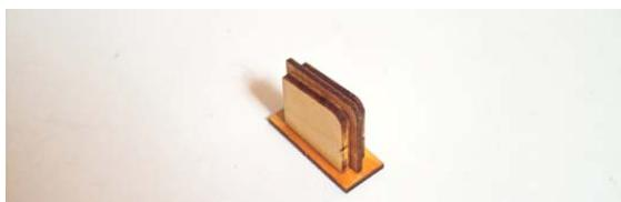
Glue the motor plate (79) to the right side as shown.
