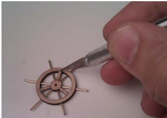
Carefully cut out the laser cut dummy spokes from the lower laser part. Then sand the wooden parts carefully.
