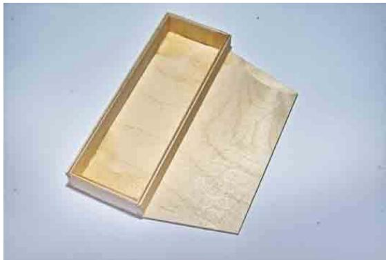
All parts for the inside of the hull should be ready now. Please varnish them 2 to 3 times and sand between, that they are water resistant. Also the deck should be varnished from the underside now.
