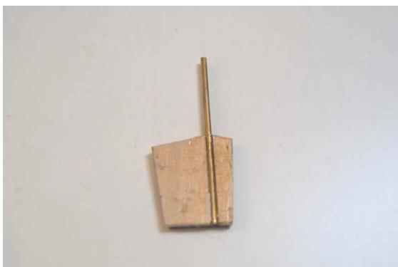
Now glue in the rudder shaft with Uhu Acrylit and the second outer plate (96 d) on top.
