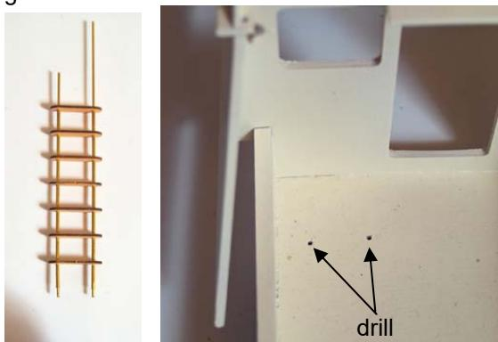
Drill the holes for the ladder at the correct place into the cockpit floor. Then bend the upper end of the longer rod at a distance of 30 mm from the highest step horizontally to the side.
