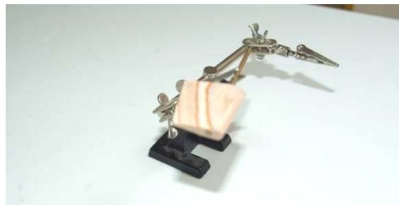
Now make a profile on the rudder, sharp at the end and round at the front.
