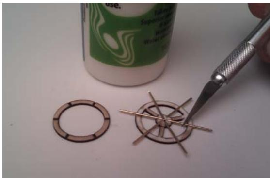
Apply some glue to the outer ring and into the center of the wheel and place the spokes carefully that they are lying up to the center hole, but leave it free.
