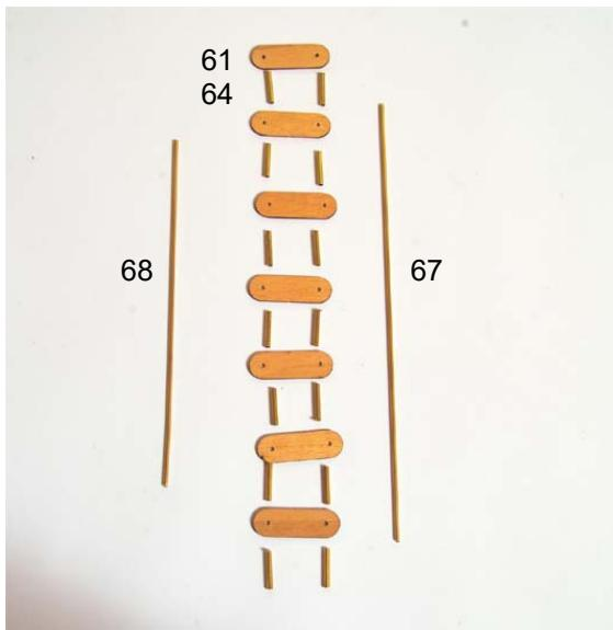
Glue the first two distance tubes 5 mm from the lower end of both vertical rods. Then place alternately one Step and two distance tubes onto the rods and fix the with a drop of superglue.
