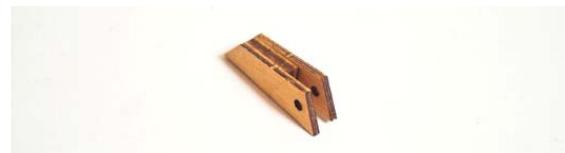
After sanding and painting place reel and pin and fix the pin with a drop of medium super glue. If necessary you have to sand down the reel on both sides to fit between the two sides.
