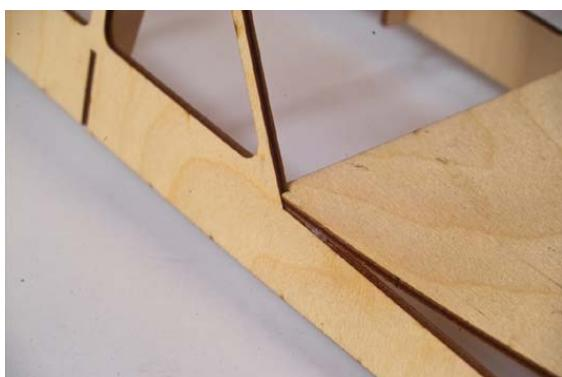
Fix the roof at its cut outs with superglue
