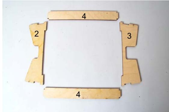
First build the boat stand with parts 2, 3 and 4. After the glue is dry carefully sand and varnish the stand several times. As you will later place your wet model on the stand, it is important to have this water resistant. As an apolster you can use some pieces of foam tape on the upper sides which will contact the hull.
