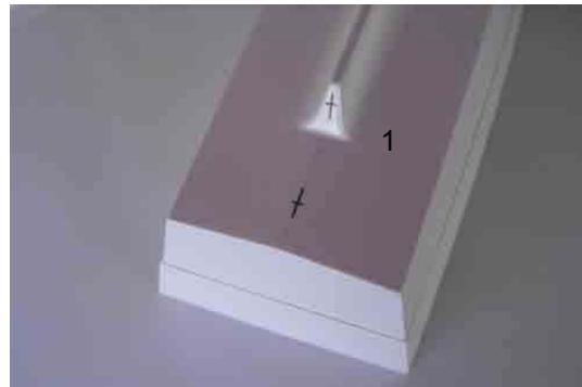
Now drill the holes for prop shaft and rudder tube.
