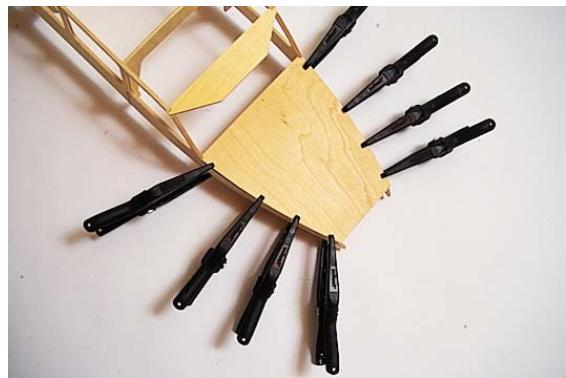
When the glue is dry, do the same on the other side. After that glue from inside and fix with clamps.
