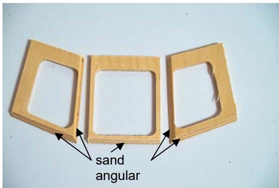
In the next step you have to sand the contour of the main roof on top of the front windows in the same way as the contours of the frame and back wall.
