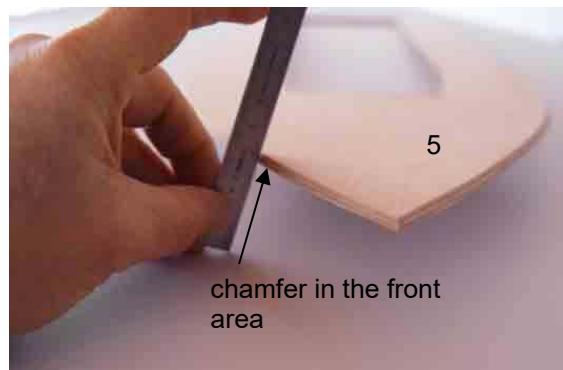
Now place the deck into the hull and mark a line on the sides 2 to 3 mm over deck level. Cut the hull down only until to this line with a sharp knife or strong scissors.
