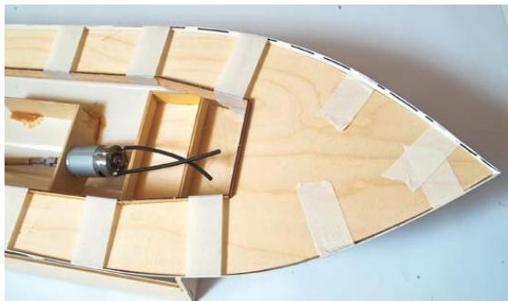
Fix the deck at several points with thin superglue. After that you can fix the deck complete
