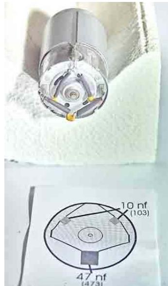
Now solder motor wires to the connections.
