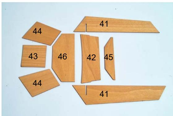
First the parts 41 and 42 will be glued together. Place strips  $3 \times 5 \times 40$  mm for strengthening.
