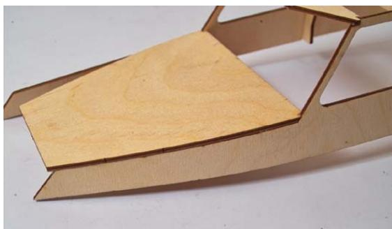
When the glue is dry, bend the side according to the curve of the roof and fix with superglue.
