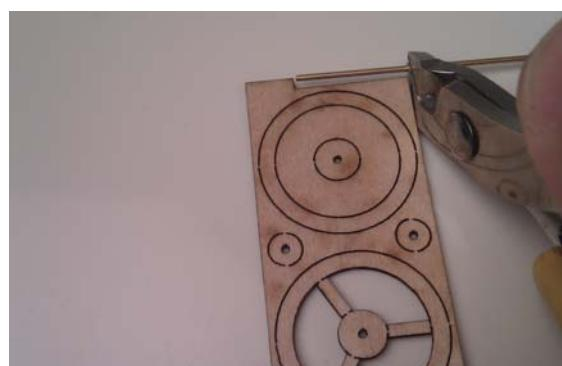
Use the cut out on the laser sheet to cut equal lengths for 6 spokes fom the brass wire 1 mm.
