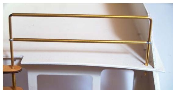
Make the end piece at the left ladder rod from a piece of brass tube 2 x 7 mm (104) and glue.
