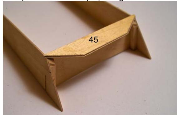
Then place the flybridge on the top of the roof, check alignment and fix with superglue. To match the curve of part 42 to the curve of the roof, you can place sand paper flat onto the roof and sand the wall to have a better fit, if necessary.
