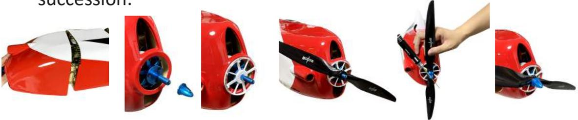
3. Secure the spinner with screws, please pay attention that spinner must be located in the centre position of the cowl, and spinner edge is parallel to the cowl, gap is about 1.5mm.
