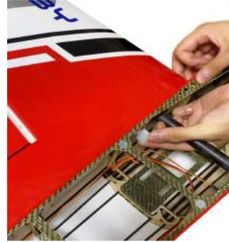
10. Unscrew the retaining screws on the wing, install wingtip.
