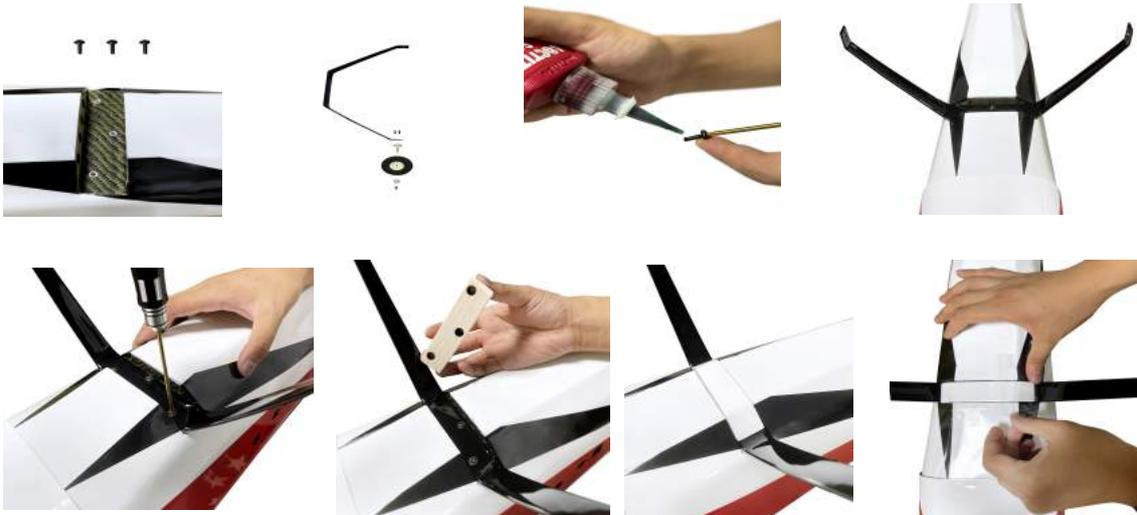
4. Install landing gear cuffs, Secure it with electrical tape.
