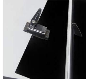
6. Secure aileron servo arm and control horns with ball head pull rod, put the cup head hexagonal screw, gasket, ball head on servo arm, secure it with iron pliers, adjust the ball head pull rods to proper length.
