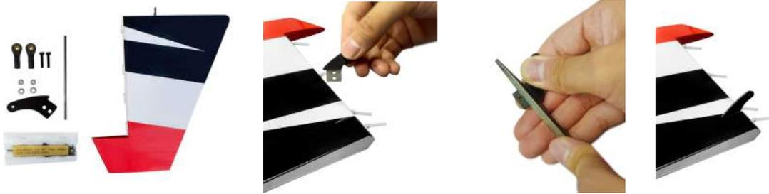
3. Remove 4 hinges which are inserted in the rudder. Inject AB glue into the holes, apply glue to 4 hinges with appropriate length from its bottom, then insert 4 hinges into the rudder.
