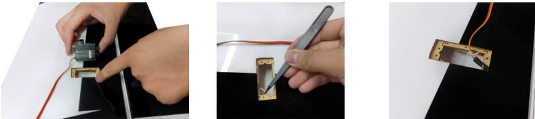
4. Find the other head of white polyester thread from wing side, pull it until aileron servo is placed in servo hole.
