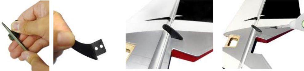
3. Remove the secured plate used for filling the horizontal tail slot, insert the horizontal tail into fuselage, please take note that it must be fully inserted into the fuselage.
