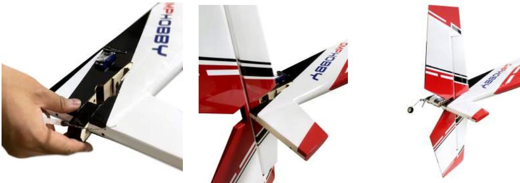
4. Insert secured plate to fill the horizontal tail slot, use 502 gluing the gap all around the horizontal tail.
