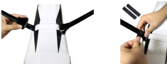
5. Install wheels, Secure wheels with gasket and screw.
