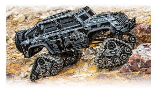
Each Traxx drive unit is engineered for rugged, yet smooth performance. An adjustable tension wheel keeps the treads tight while suspended road wheels allow the tread to conform to surface irregularities for maximum traction. Oil-filled dampers on each drive unit control rotational movements to help keep the tread glued to the surface. The rear Traxx drive units are longer to allow climbing steeper grades with authority.
