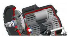
ratio for dirt-slinging speed. When the terrain turns technical, drop it into "low range" for a 70:1 ratio and unreal climbing torque. For the ultimate in climbing traction, flip the T-Lock switch to lock the front differential. Need even more grip? Activate the rear T-Lock diff for fully-loaded 4WD power no matter which tire is gripping or slipping.
