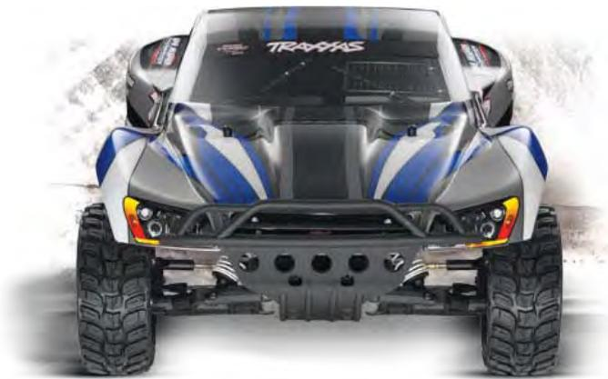
**MODEL 58024:** Fully assembled, Ready-To-Race®, with TQ™ 2.4GHz radio system, waterproof XL-5 Electronic Speed Control, Titan 12-turn motor, and ProGraphix® painted body.
