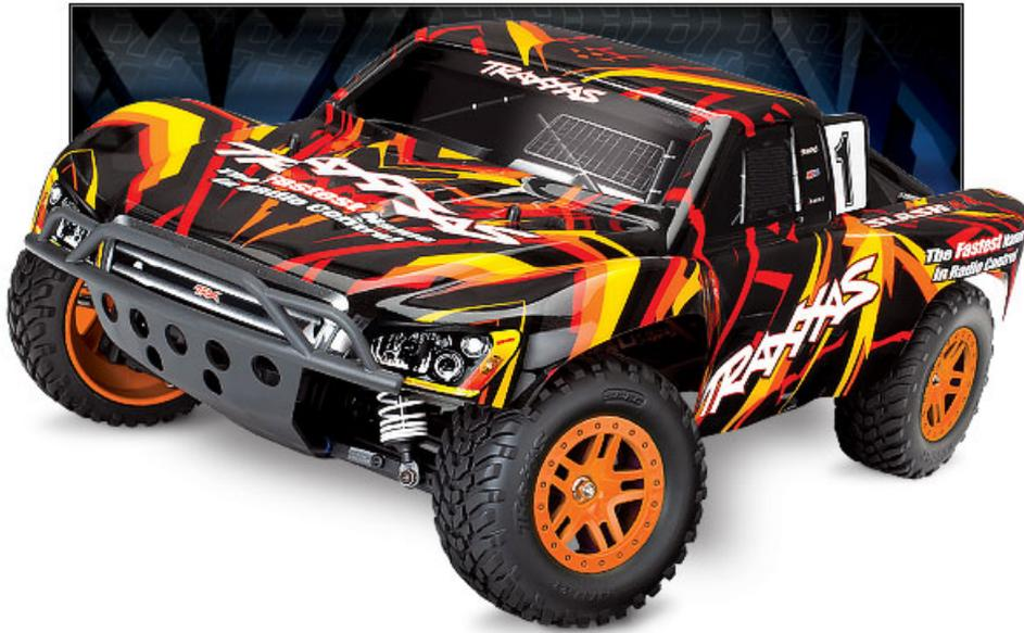
**MODEL 68054-1:** Fully assembled, Ready-To-Drive®, TQ 2.4GHz Radio System, XL-5 electronic speed control, 4-amp DC Peak Detecting Fast Charger, 7-cell NiMH battery with iD™, and ProGraphix® painted body.
